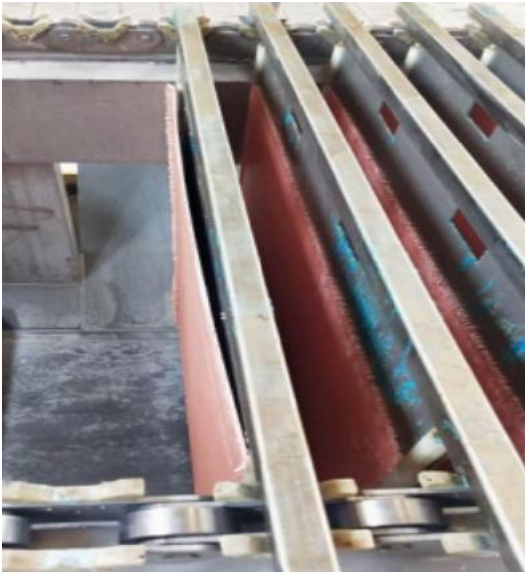
Picture 1. Copper Cathode Formation Without Proper Clean of the Cathode
